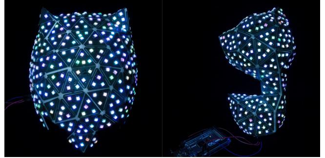
Fig. 8. *batman* and *cat* model fabricated with big LEDs using the maximal density of our placement algorithm.
